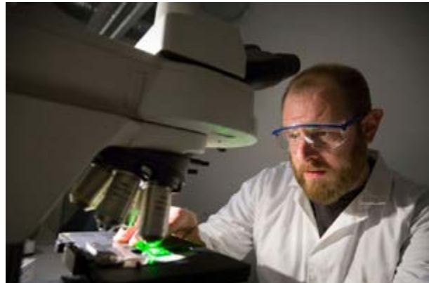
Dr Andy Booth using fluorescence microscopy to identify microplastic particles in environmental samples.
