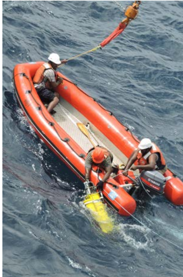
Recovery of a Lagrangian Float that is used to study the top uniform layer of the ocean
