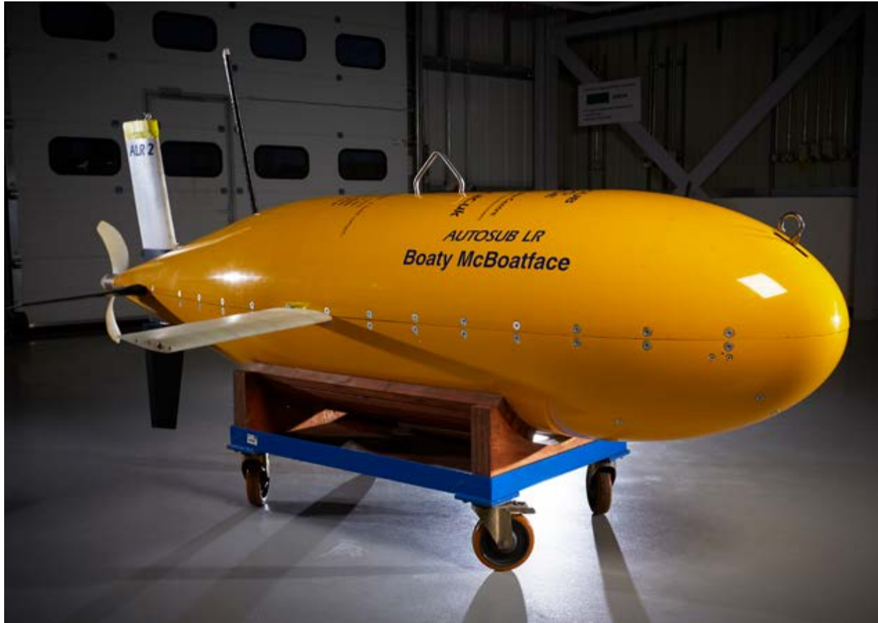
Boaty McBoatface – one of the National Oceanography Centre’s autosubs – a long range autonomous vehicle that can travel for many kilometres and to great depths underwater, gathering scientific data.
