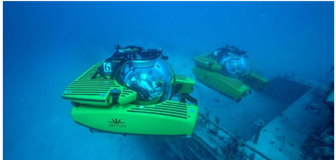
Triton: a three-person ocean research vessel with a diving depth of 2300m that will be used by researchers on REV I. Photo: REV Ocean
